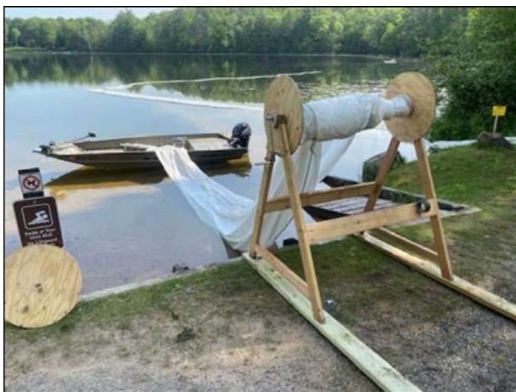
Figure 37: Limno-curtain material on a roll before installation (photo from Marinette Co. LWCD)
